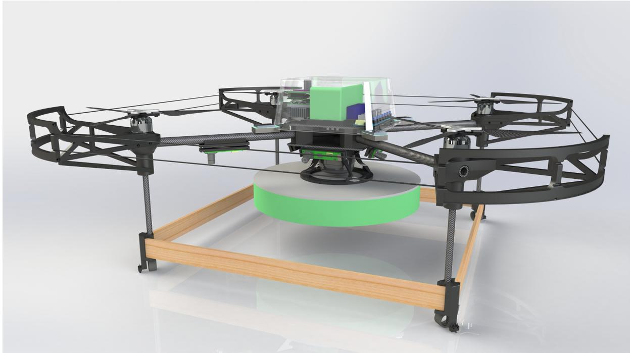
*Figure 4. Render of our drone's CAD model*
